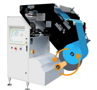
Replacement roll auto-rotates to replace empty spindle.
